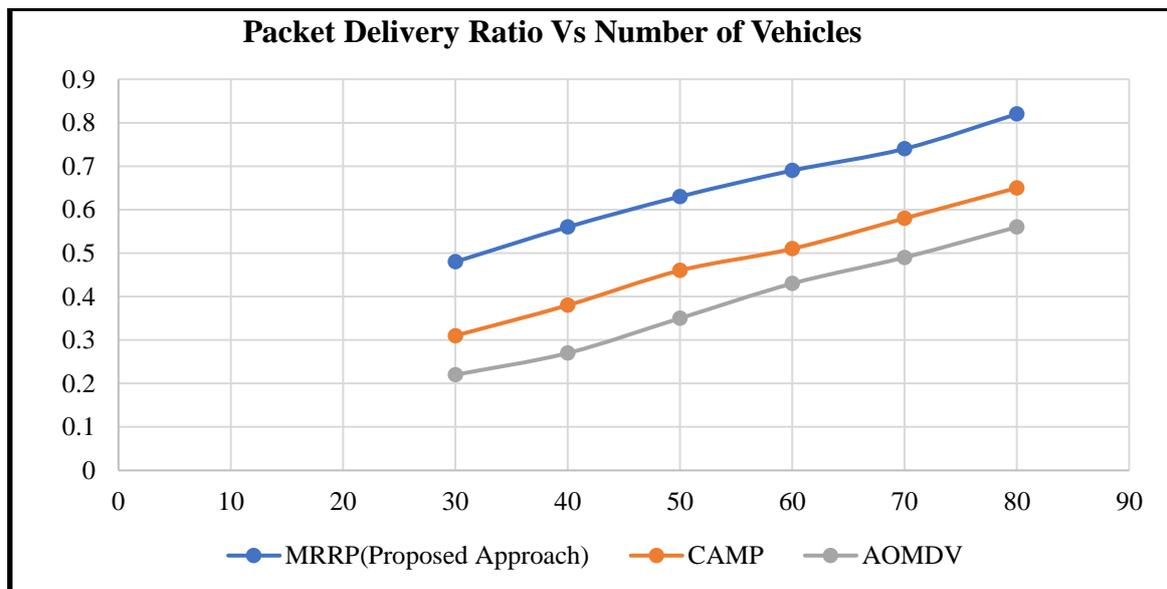
**Figure 5.** Packet Delivery Ratio (PDR) Vs Number of Vehicles
