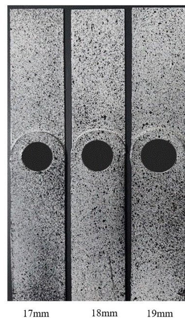
Figure 4. Speckle Pattern Applied on SLJ Specimens
