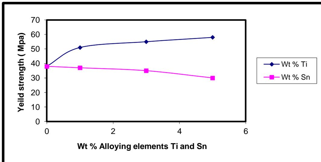
Figure (12): Effect of Ti and Sn additions with different percentages (1, 3, and 5) wt % on the Yield Strength (in Mpa) of Al-6.9%Si-1.7%Cu alloy.
