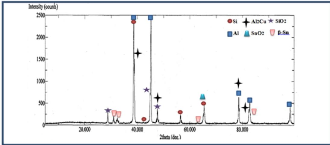
**Figure (7):** The results of x-ray diffraction for (Al-6.9%Si-1.7Cu) alloy after adding 3 wt% Sn
