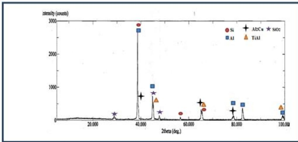
Figure (4): The results of X – ray diffraction for (Al-6.9%Si-1.7%Cu ) alloy after adding 3 wt% Ti
