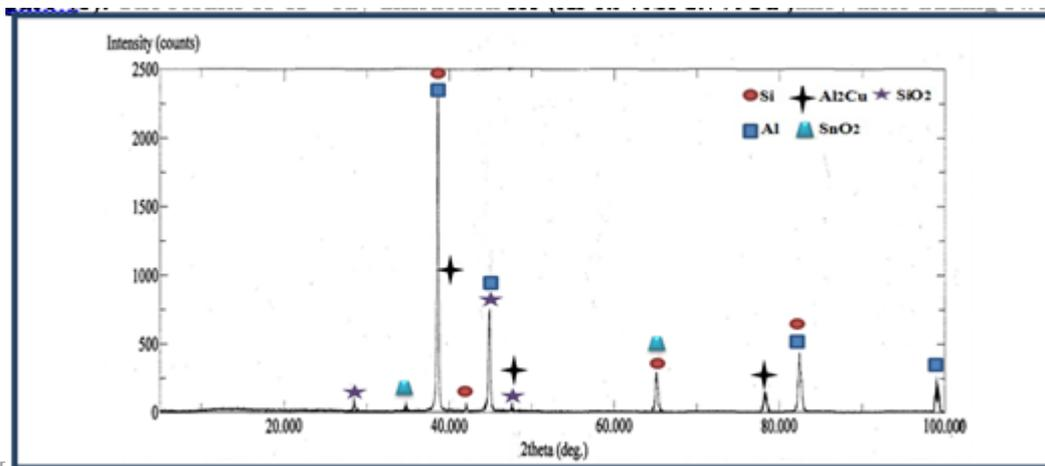
**Figure (6):** The results of x-ray diffraction for (Al-6.9%Si-1.7Cu) alloy after adding 1 wt% Sn.
