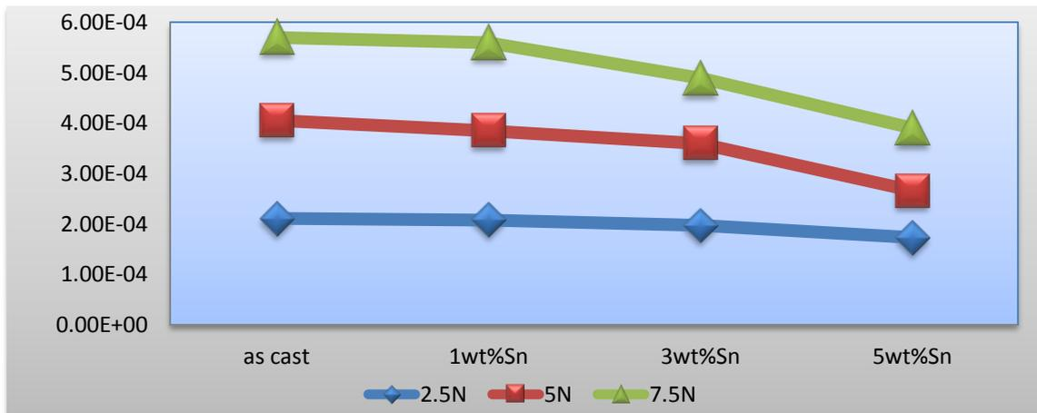
Figure (17): Effect of 1%, 3% and 5%Sn additions on wear rate of Al-6.9%si- 1.7%Cu
