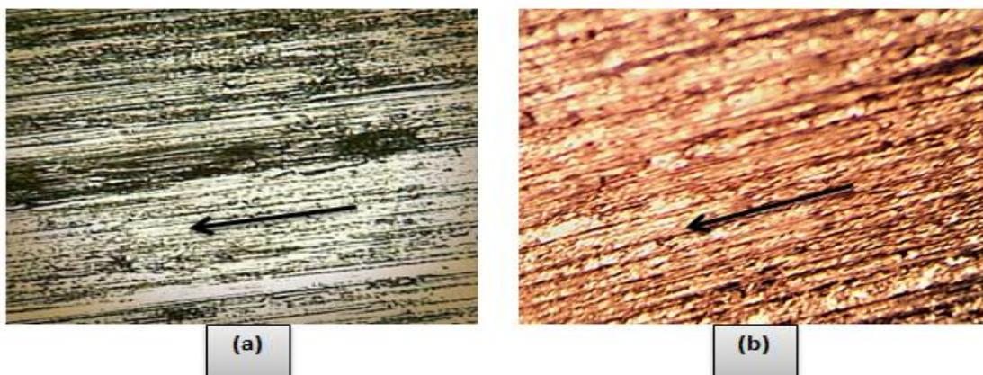
Figure (19): Optical micrographs of the surface topography of different worn surfaces under low and high loads of (2.5 and 7.5)N and under dry sliding conditions for Al-6.9Si-1.7%Cu - 3%Sn alloy, a- 2.5N, b- 7.5 N .Mag .125X.
