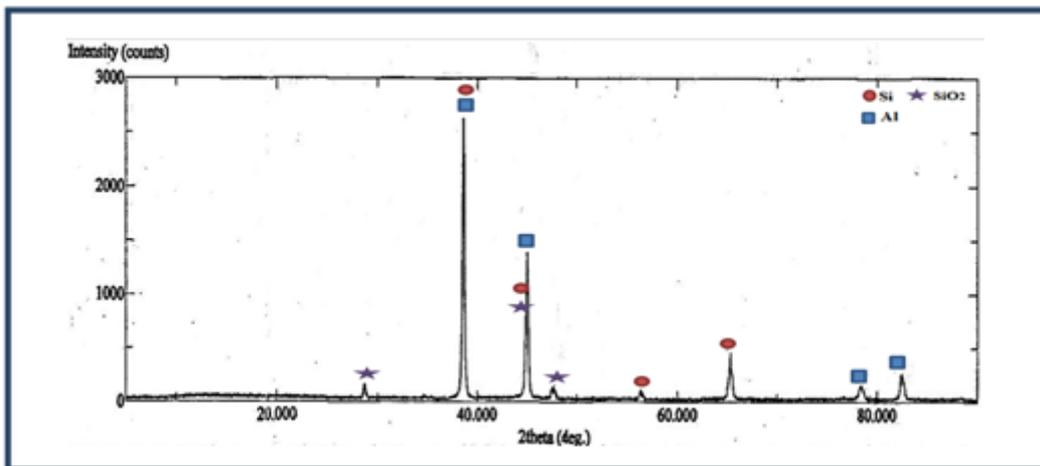
Figure (2): The results of x-ray diffraction for the base alloy (Al-6.9%Si-1.7%Cu) alloy
