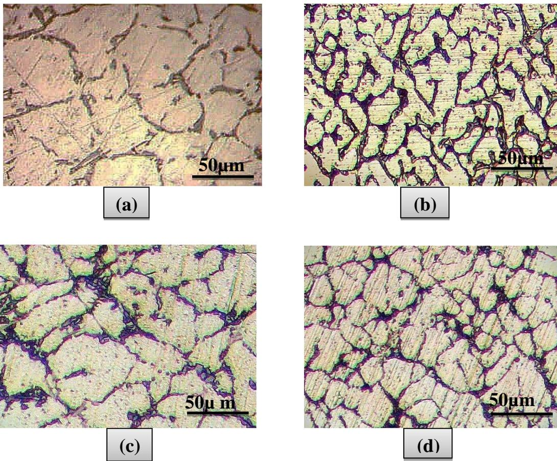
**Figure (10):** Optical micrographs of Al-6.9%Si-1.7%Cu and Al-Si-xSn alloys. (a) Al-6.9Si-1.7Cu, (b). Al-6.9Si-1.7Cu-1Sn, (c) Al-6.9Si-1.7Cu-3Sn, (d) Al-6.9Si-1.7Cu-5Sn.
