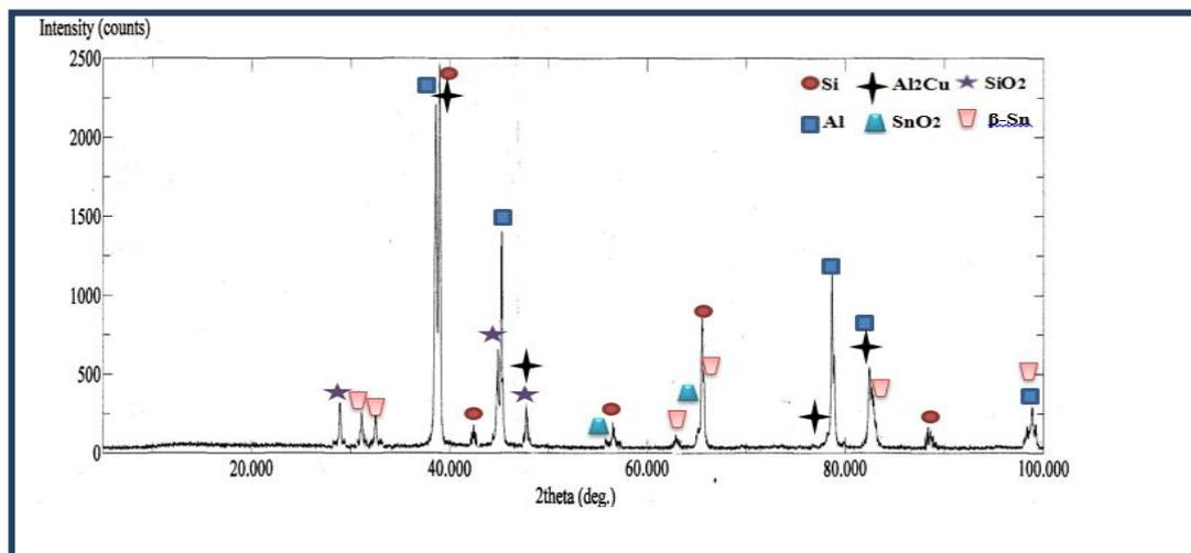
**Figure (8):** - The results of x-ray diffraction for (Al-6.9%Si-1.7Cu) alloy after adding 5 wt% Sn.
