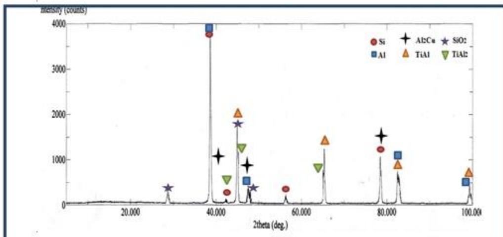
Figure (3): The results of X – ray diffraction for (Al-6.9%Si-1.7%Cu) alloy after adding 1 wt % Ti.
