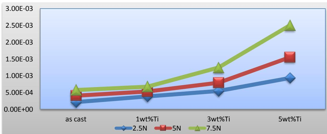
**Figure (16):** Effect of 1%, 3% and 5%Ti additions on wear rate of Al-6.9%Si- 1.7%Cu.
