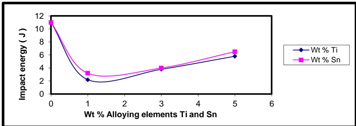
**Figure (15):** Effect of Ti and Sn additions with different weight percentage (1, 3 and 5)wt% on the impact energy of Al-6.9%Si-1.7%Cu .
