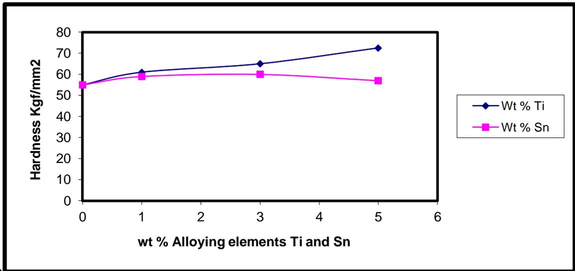
**Figure (14):** Effect of Ti and Sn additions with different percentages (1, 3, and 5) wt% on the macrohardness of Al-6.9%Si-1.7%Cu alloy
