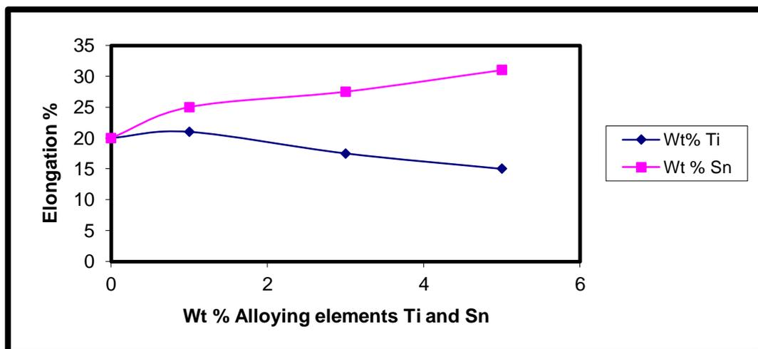
.Figure (13): Effect of Ti and Sn additions with different percentages (1, 3, and 5) wt % on the Elongation of Al-6.9%Si-1.7%Cu alloy .
