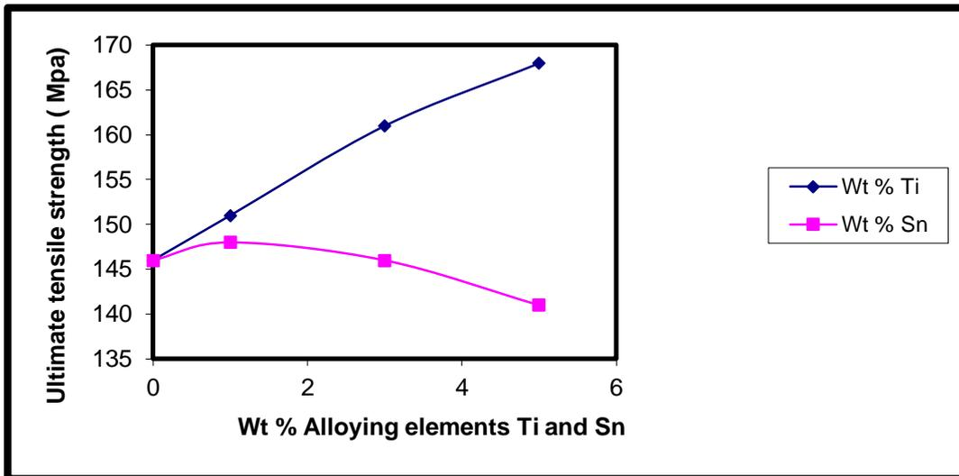
Figure (11) : Effect of Ti and Sn additions with different percentages (1, 3 ,and 5) wt% on the Ultimate Tensile Strength (in Mpa) of Al-6.9%Si-1.7%Cu alloy.
