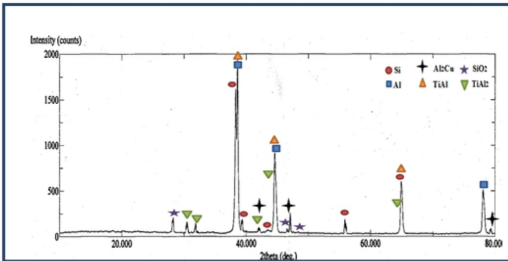
. Figure (5): The results of X – ray diffraction for (Al-6.9%Si-1.7%Cu) alloy after adding 5wt% Ti
