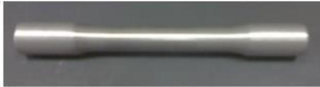
Figure (1): Standard tensile test specimen
