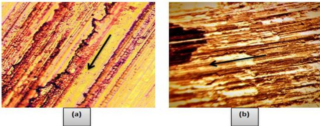
Figure (18): Optical micrographs of the surface topography of different worn surfaces under low and high loads of (2.5 and 7.5)N and under dry sliding conditions for Al-6.9Si-1.7%Cu - 3%Ti alloy, a- 2.5N, b- 7.5N, Mag.125.
