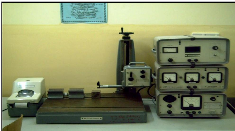
Figure (3) Roughness measuring apparatus.
