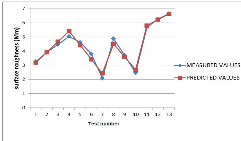
Figure (4) Relationship between measured and predicted Ra (coated wire).
