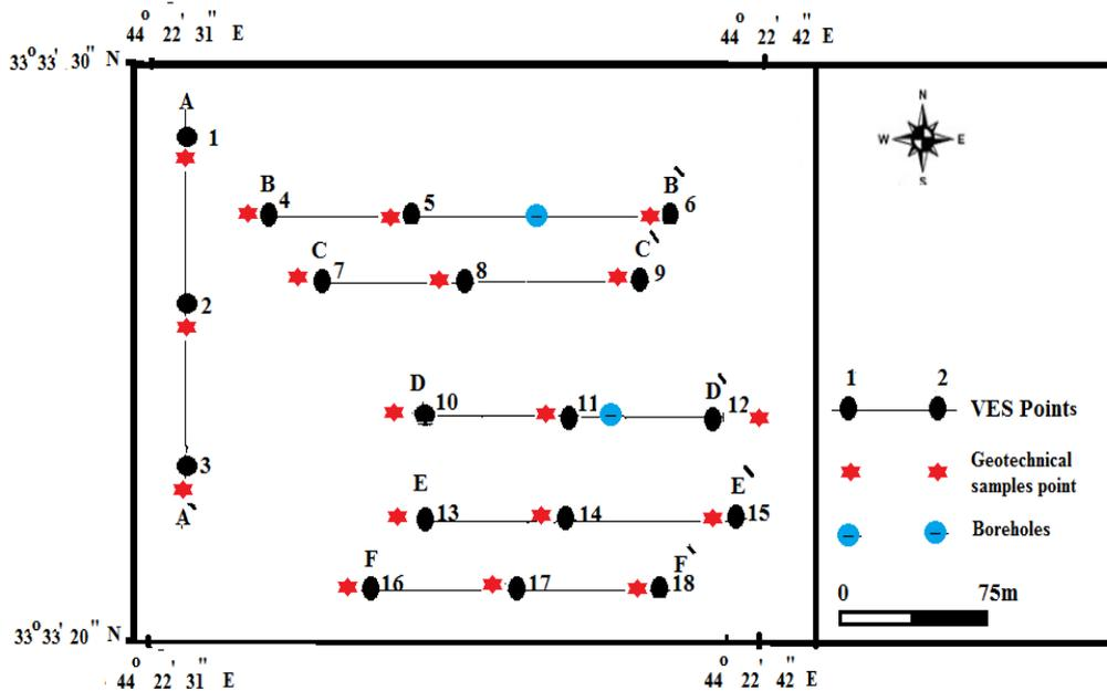
Figure (3) Data Acquisition Map of the Study Area Showing the Vertical Electrical Sounding Stations and the Geotechnical Sampling Points
