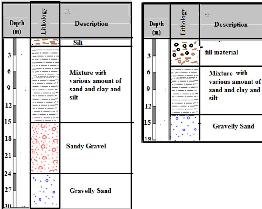
Figure (2) Soil section in B.H.1, B.H.2 in the study site after NCCL2000 (modified)
