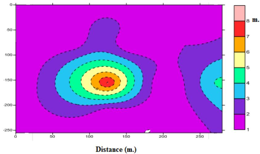
Figure (8) Isopach Map of the Topsoil.
