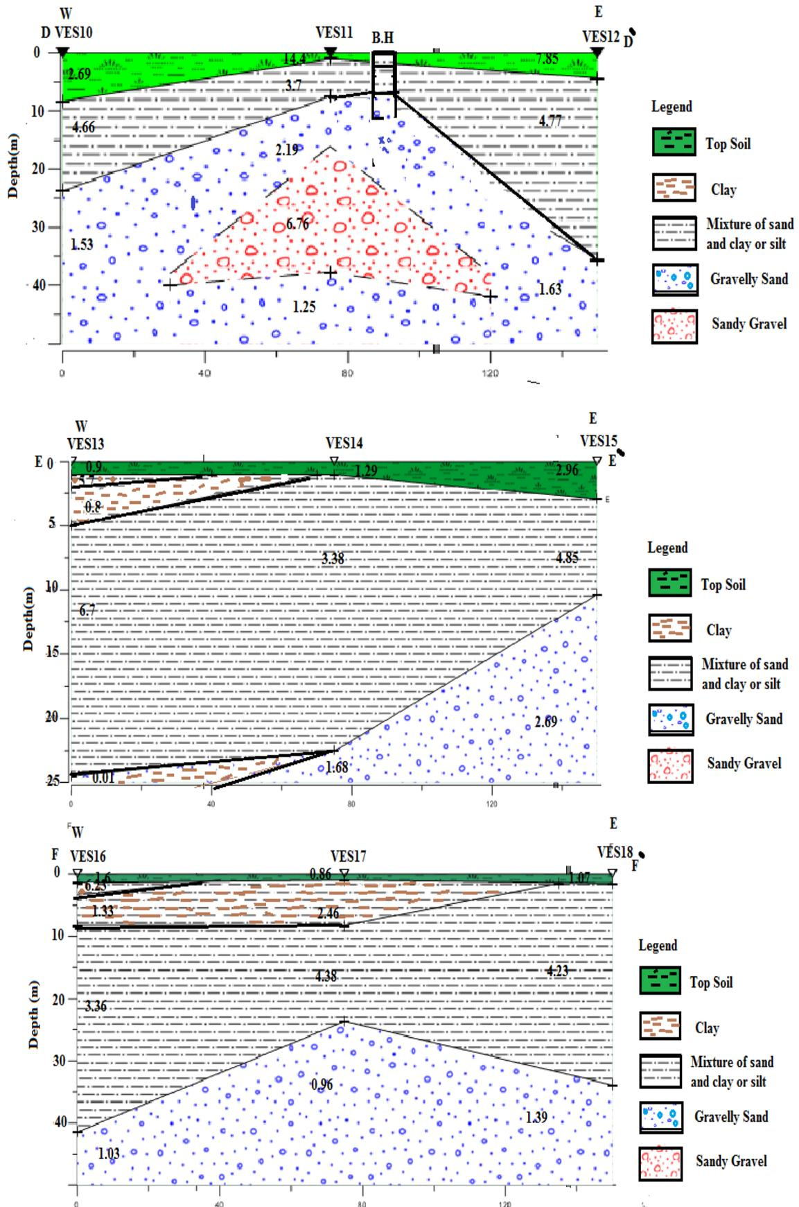
Figure (6) Geoelectrical cross section along profiles DD', EE', and FF'
