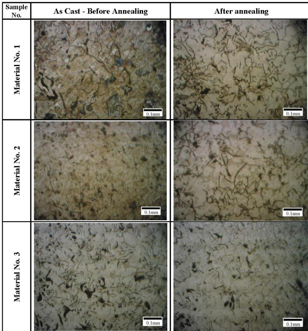
**Figure (4):** Microstructure of material No. 1, 2, & 3 before and after anneal.
