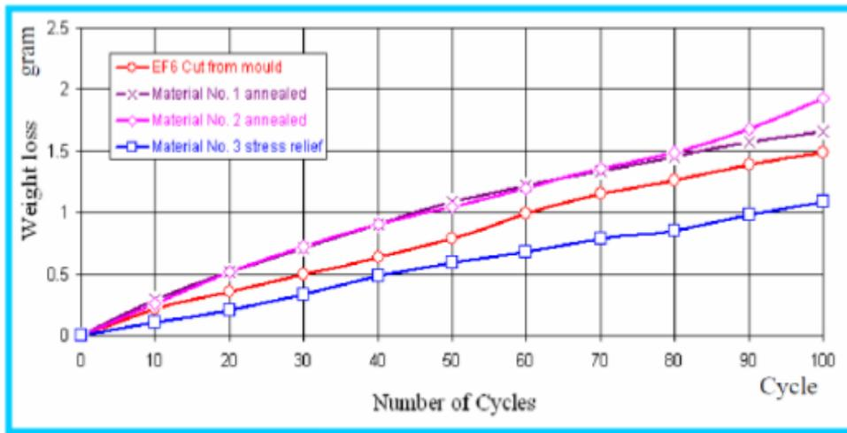
Figure (12): Average Weight loss (gram) as a function of number of cycles for heat treated materials (After full annealing) tested at 850°C.
