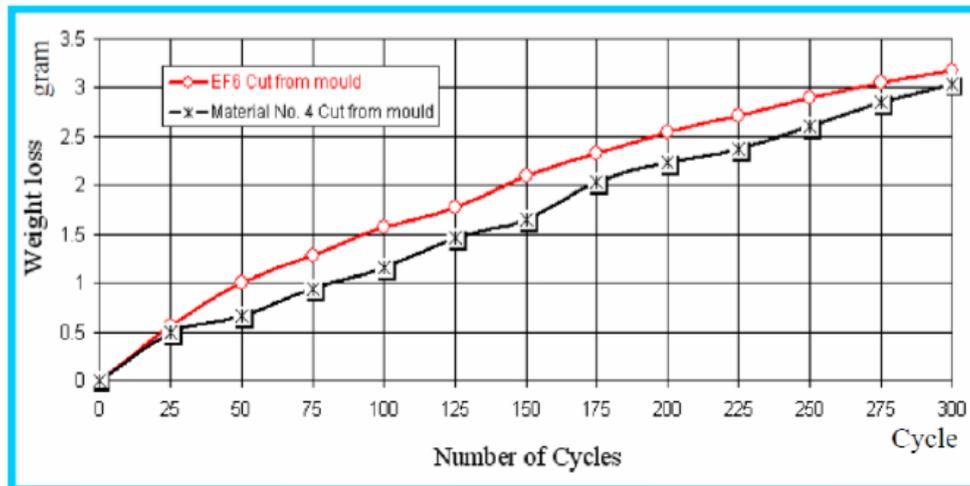
Figure (13): Average Weight loss of material No. 4 compared with EF6 material as a function of number of cycles for as-cast condition tested at 600°C.
