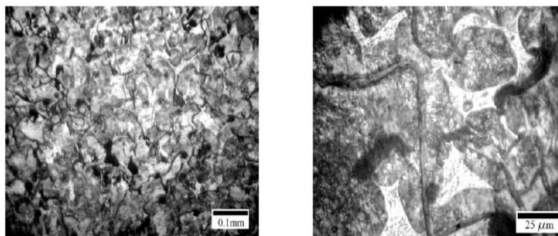
**Figure (5):** Microstructure of material no. 4 (as cast condition without heat treatment).
