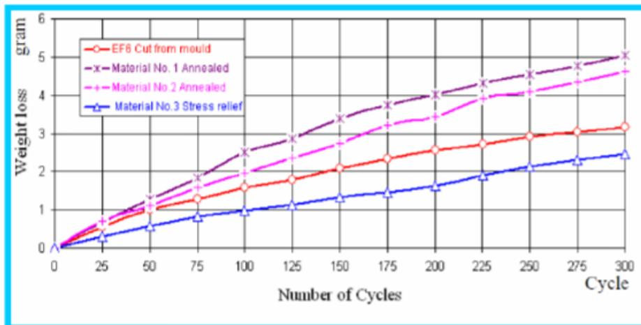
Figure (10): Average Weight loss (gram) as a function of number of cycles for heat treated materials (After full annealing) tested at 600°C.
