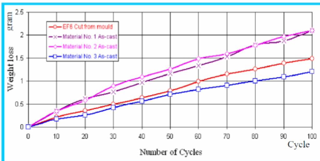
Figure (11): Average Weight loss (gram) as a function of number of cycles for as-cast materials (Before annealing) tested at 850°C.
