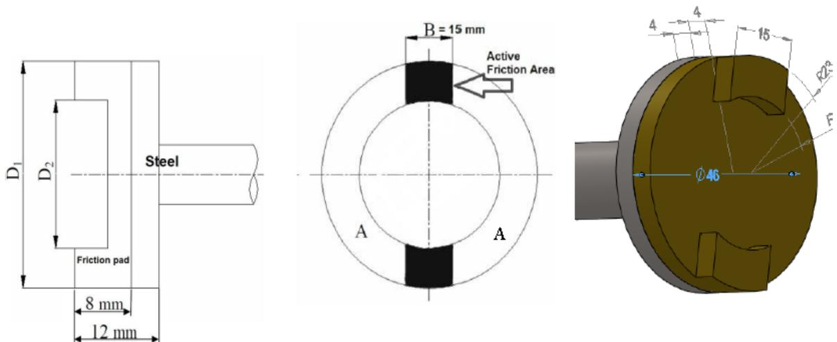
Fig. 8. The friction material Pad
