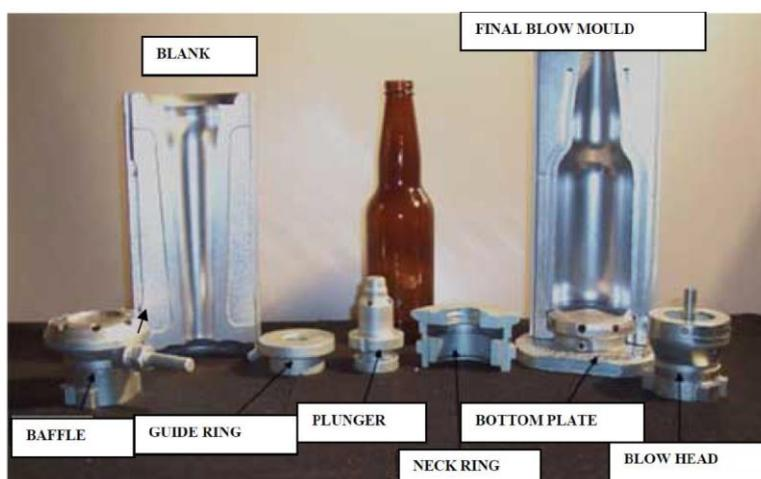
**Figure (1):** Glass blow mould parts <sup>(13)</sup>.
