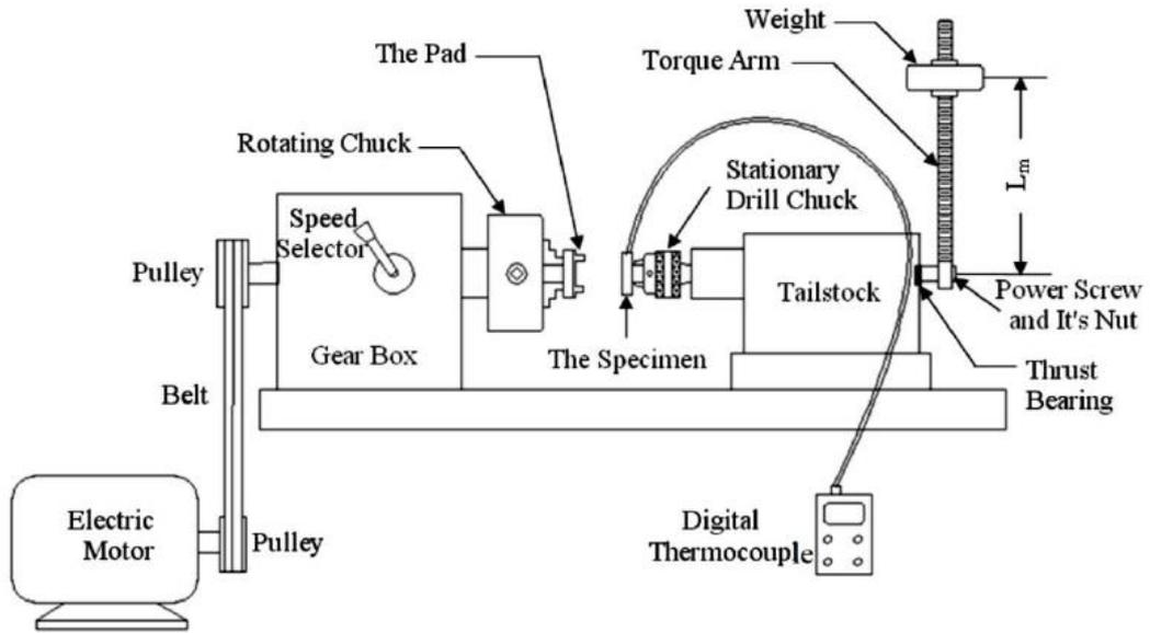
Fig. 6. Schematic diagram of the wear tester
