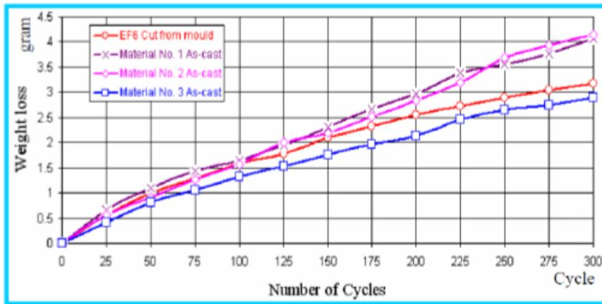
Figure (9): Average Weight loss (gram) as a function of number of cycles for as-cast materials (Before annealing) tested at 600°C.
