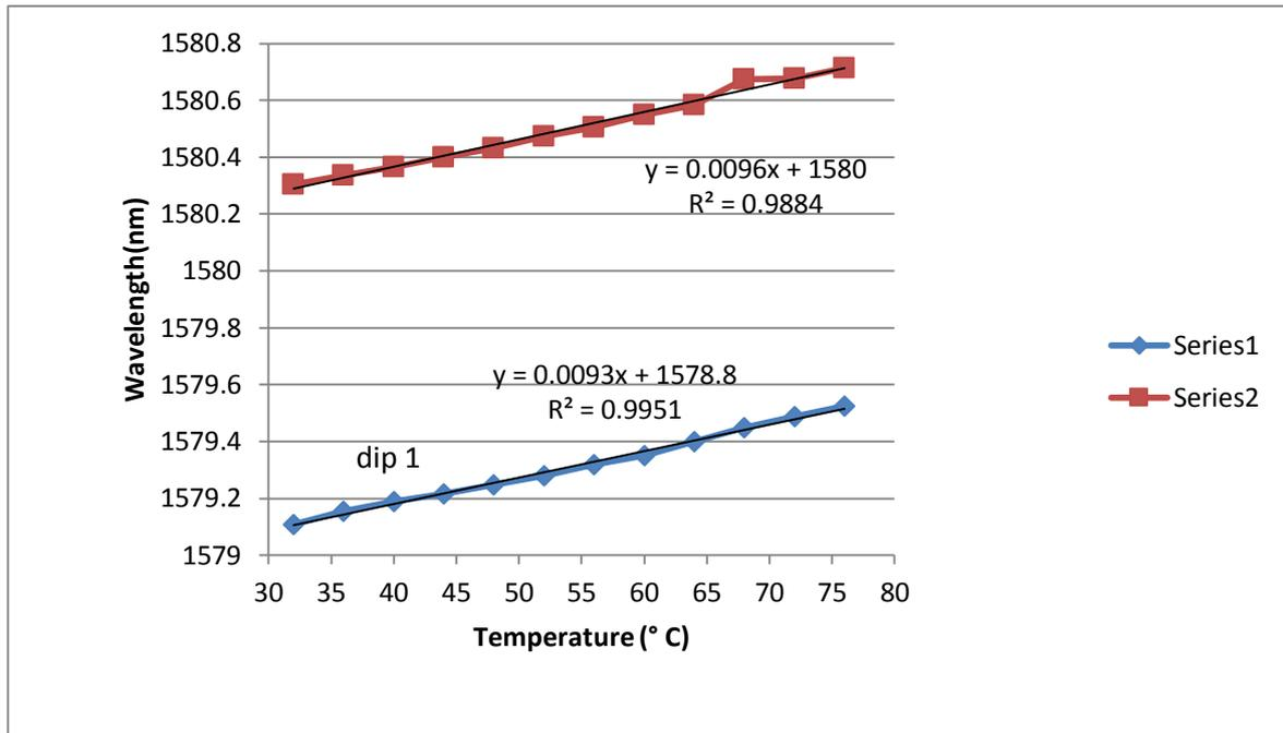
Figure (5): The relationship between temperature and wavelength of the second TFBG.
