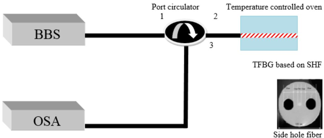
**Figure (1):** A schematic diagram of the sensing system involving the home made tilted fiber Bragg grating
