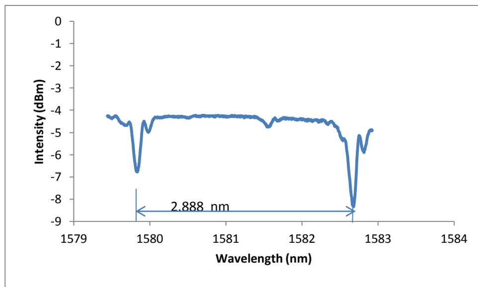
**Figure (2):** Transmission spectrum of the TFBG written on 7cm side hole fiber.
