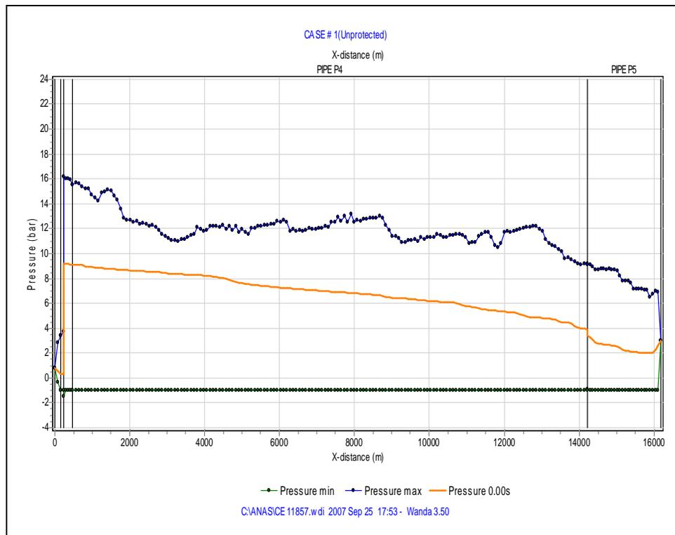
Fig.(5): Pressures along pipeline for Case #1 (unprotected).
