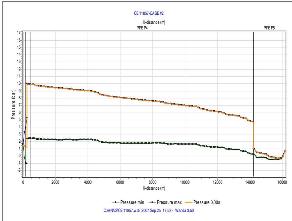
**Fig.(8):** Pressures along pipeline for Case #2 (protected).
