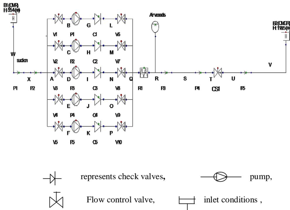
Fig.(4): shows a simplified scheme for the system components and nodes.
