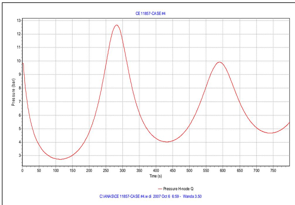
**Fig.(11):** Pressure at delivery side of pump station for Case #4.
