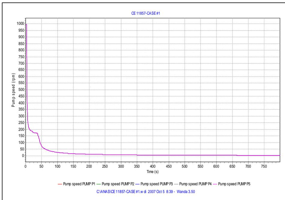
**Fig.(7):** illustrates the 5 Pumps speed changes after tripping (CASE #1).
