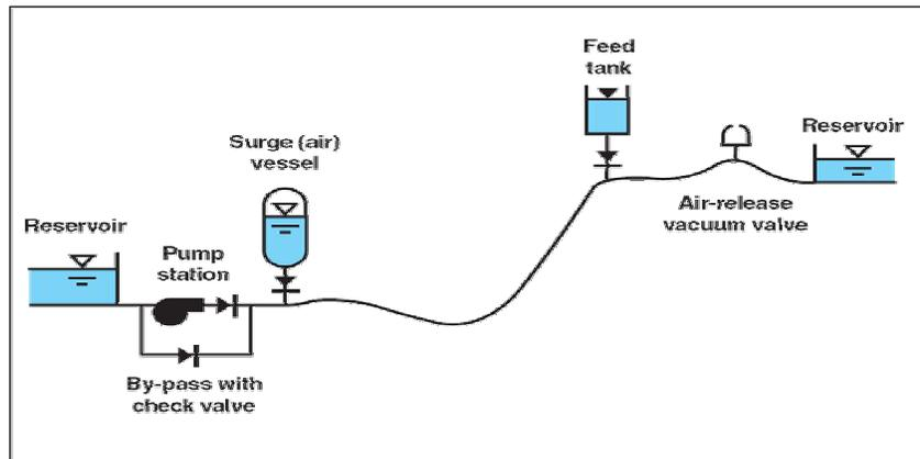
**Fig.(1):** typical locations for various surge protection devices.
