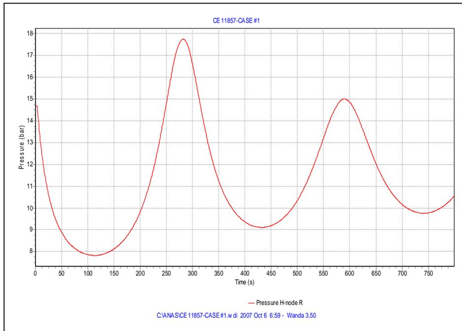
**Fig.(6):** Pressure at Node (R) for Case #1 (unprotected).
