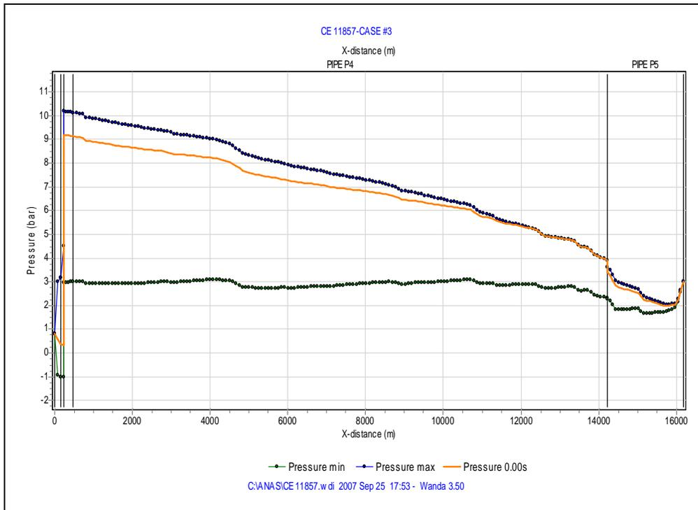
**Fig.(10):** Pressures along pipeline for Case #3 (protected).
