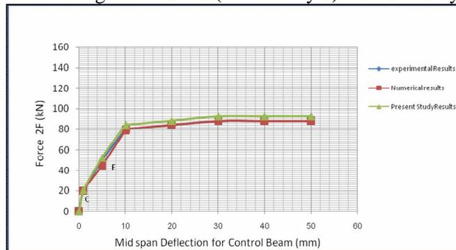
**Fig.(14):**Load- Deflection Curves for Control Beam(Case Study 1).
