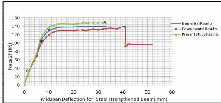
Fig.(16): Load- Deflection Curves for Beam Strngthened with Steel Plate(Case Study 1).
